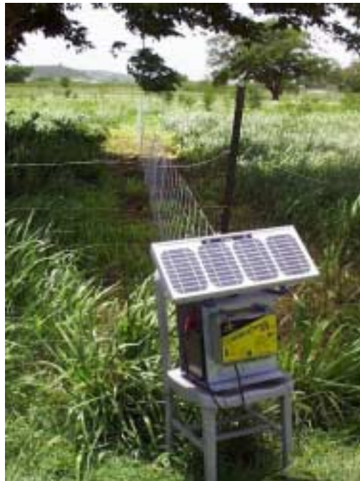
Figure 2. Electric fence powered by solar panel and a battery. The fence is easily moved to partition sections of the pasture.
