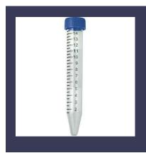
Centrifuge tube: Use this tube to collect a water sample from your sink faucet (fill to  $\sim 10 - 12$  ml).
