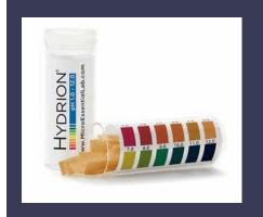
pH Test: Insert litmus paper strip into water for ~5 seconds. Compare color of strip to pH chart found on vial.
